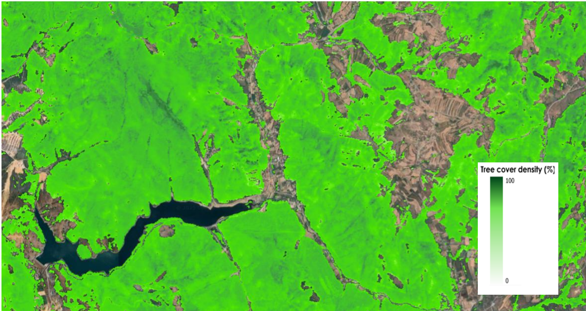
Figure 15. Classification of forest cover density by Tree Cover Density (TCD). Spatial distribution of tree crown density (%), based on the Copernicus Tree Cover Density product (10 m resolution). Source: Copernicus Land Monitoring Service (CLMS), elaborated by the authors.
